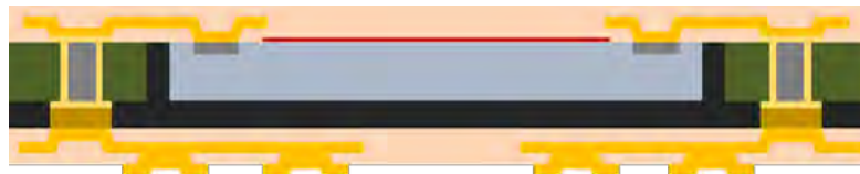
Via-Frame Fan-Out WLP (VF-FOP) with Double-side RDL
