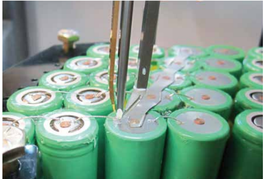
Figure 1. Process tooling – end effector, cutter, and clamp.
