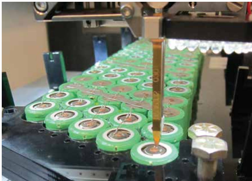
Figure 3. Close up of wire bond envelope – initiating first bond.
