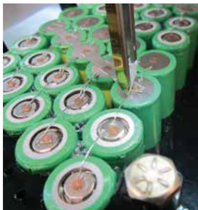
Figure 4. Aluminum wire on aluminum and nickel finishes.
