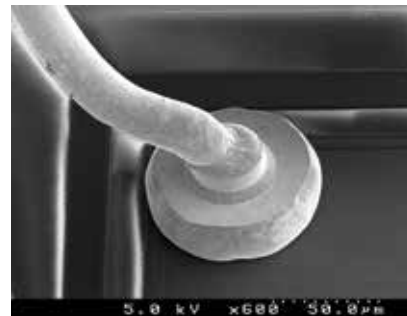
Fatigued/Deformed Wire Bond.
