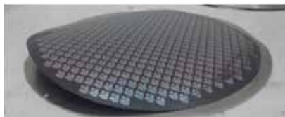
Figure 4. Example of serious warpage of reconstituted wafer.
