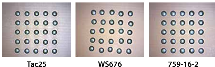
Figure 10. Sphere movement during reflow test.
