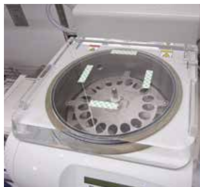
Figure 3. Vacuum centrifuge used to remove bubbles before dispense.
