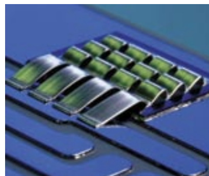
Orthodyne's PowerRibbon™ is the most advanced interconnect alternative for small SO8, PQFN type lead frame applications.
