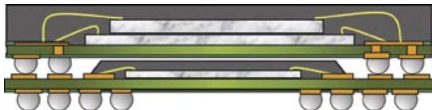
Figure 2 – Amkor's package-on-package (PoP).
