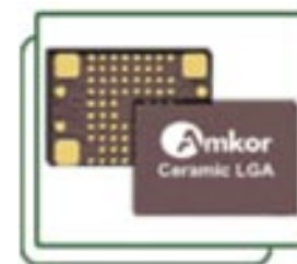
Figure 1 – A ceramic LGA package.
