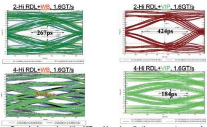
By replacing a wire with a ViP and keeping all other parameters equal (including RDL), the above performance is achieved. ViP's work at DDR3
