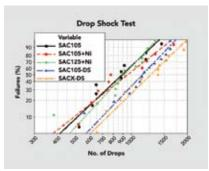
Figure 1. Drop Shock test results using 0.30mm (12mil) spheres attached to CABGA84 substrate with NiAu pad finish.
