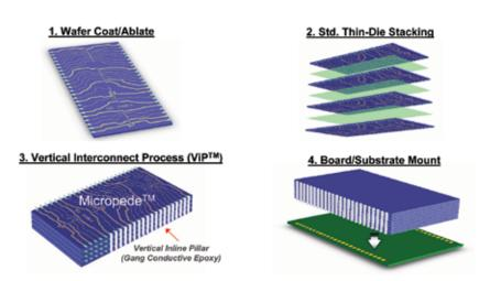
Die stacks can be built as Micropedes and surface mounted, or built "On Board".
