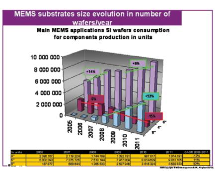
Figure 4. Evolution of the silicon MEMS substrate use in production.
