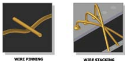
Figure 7. Examples of future layouts of insulated bonding wire, defined as wire pinning and stacking.
