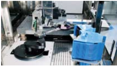
Figure 2. View of tool with robotic handling, cassettes and non-contact prealigner.
