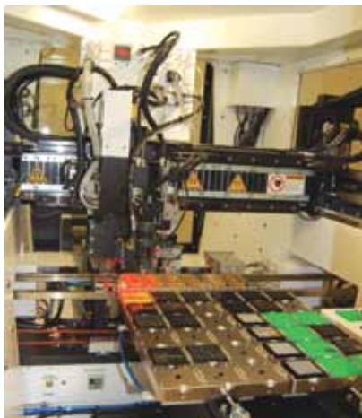
MRSI-M5: At work using tool changing capability for multiple die attach, filters, molytaps, and passives.
