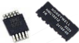
3-axis compass: X/Y: 3x3x1mm Z: 10x1.4x3.9
