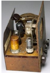
Early PCB demo in a radio.
