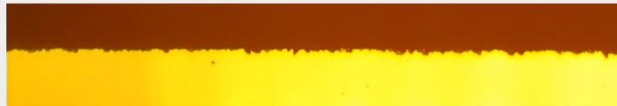
Edge as viewed from top of die (optics magnification 200x)
