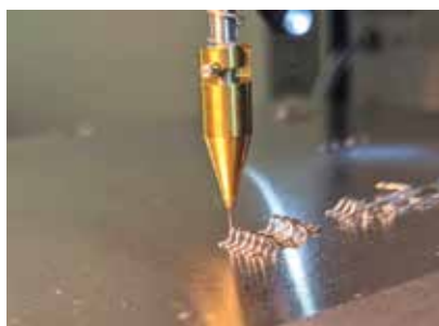
Destructive wire bond pull test in process.
