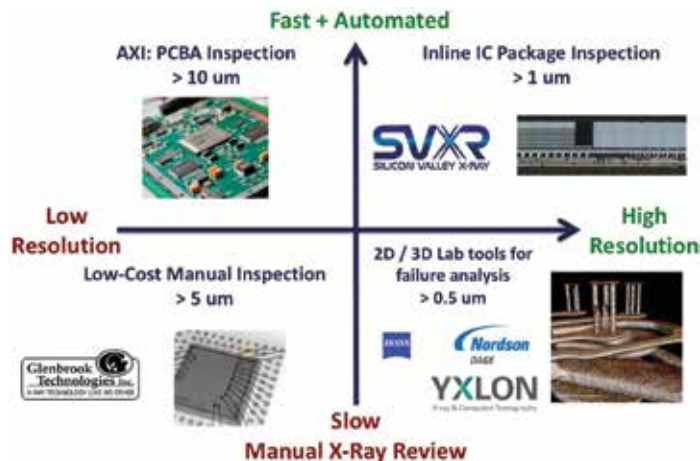
Figure 3. Four types of x-ray systems. Inline inspection for advanced IC packaging requires both high resolution and high speed imaging.
